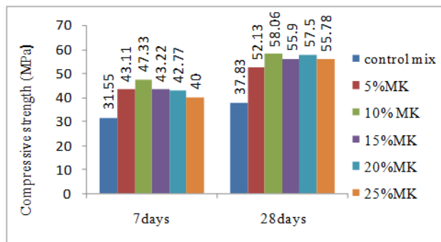
Figure 3: Comparison of Compressive Strength for Replacement by Metakaolin
